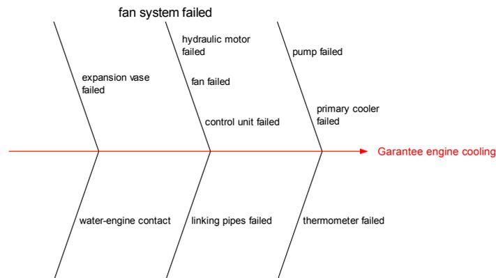
Figure 4 – Fishbone Diagram of the cooling system
