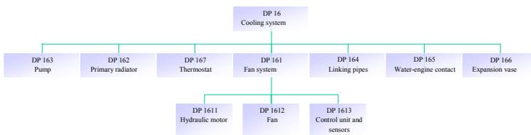
Figure 3 – AD Representation of the cooling system, DPs tree
