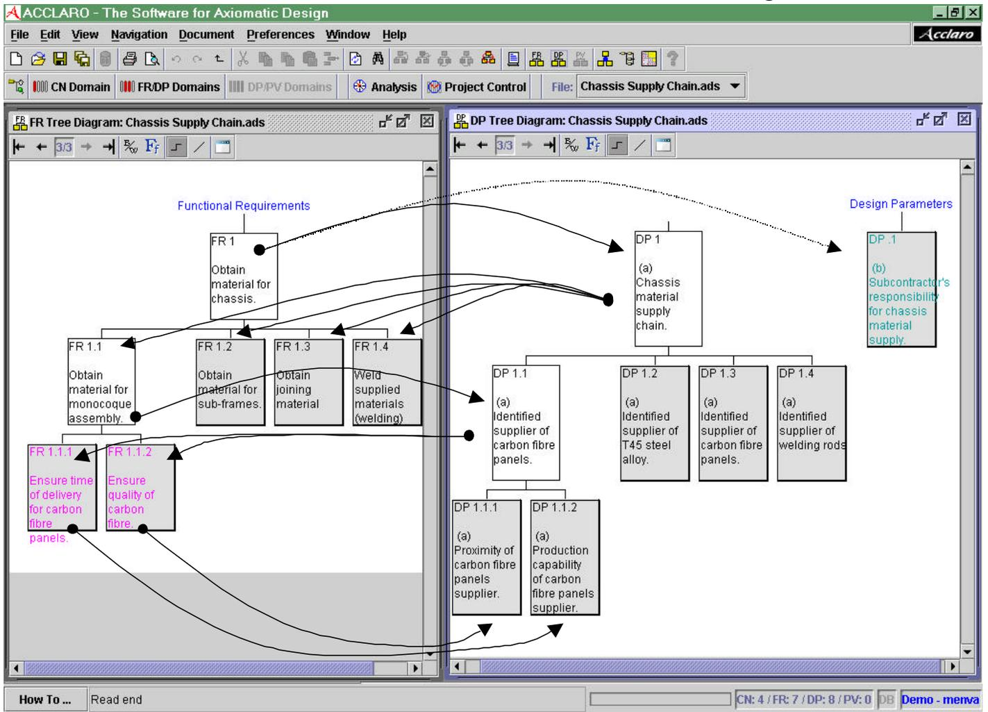
Figure 2. Car chassis supply chain FR and DP hierarchies defined in Acclaro software
