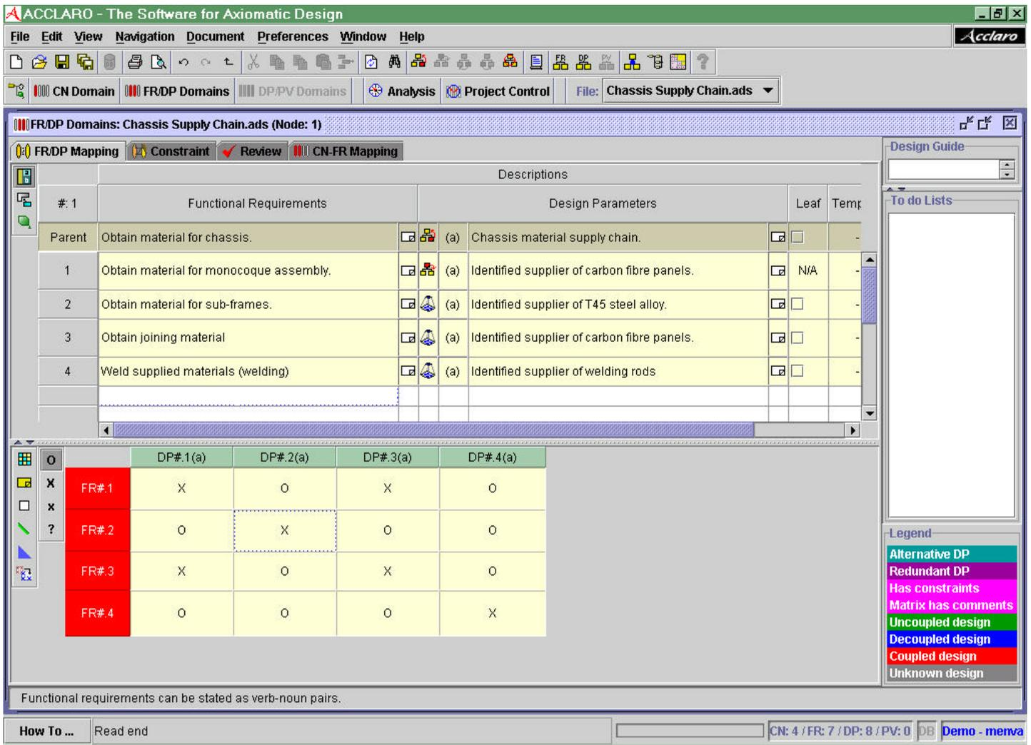
Figure 3. Car chassis supply chain design equation for the second level of FR and DP hierarchy
