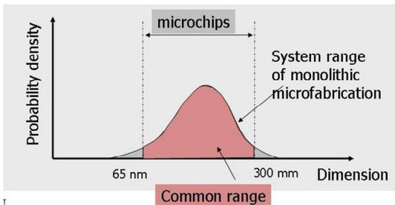
**Figure 2** The monolithic idea could make the system range of microprocessor manufacturing overlap well with the design range with the 12 inch wafer processing capability and the minimum feature size of 65 nm.
