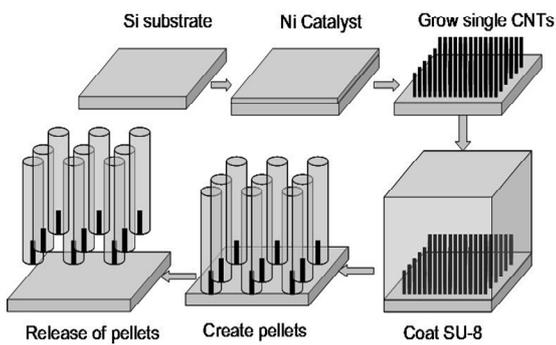
**Figure 7** Additive nanopelleting processes.
