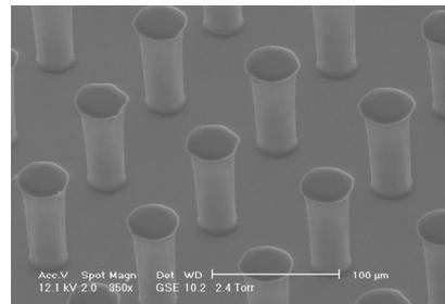
**Figure 8** High aspect ratio polymer pellets formed on the patterned nanodots.
