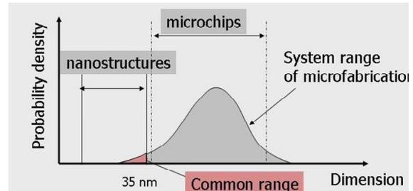
**Figure 3** The system range of microfabrication processes has very little overlap with the design range of the assembly of nanostructures.
