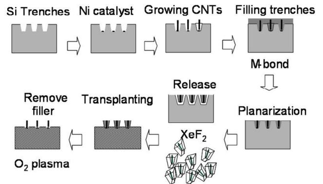
**Figure 5** Subtractive nanopelleting processes.
