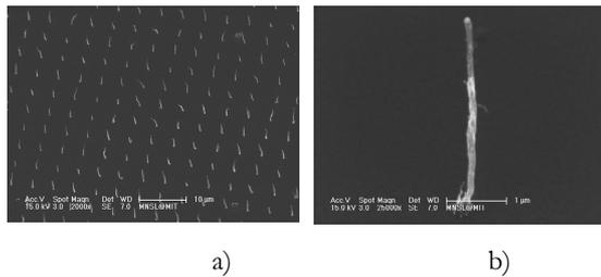
**Figure 6** Single stranded CNTs grown vertically on patterned metal nanodots (a), a close up view (b)
