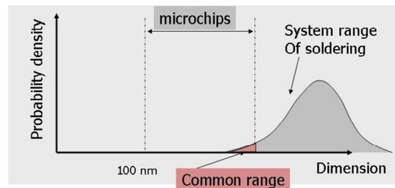
**Figure 1** System range of the manual assembly of discrete parts has very little overlap with the design range of assembling microchips.
