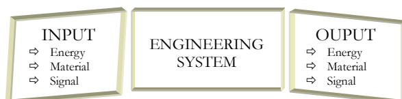
Figure 1 – The conversion of energy, material and signal.
