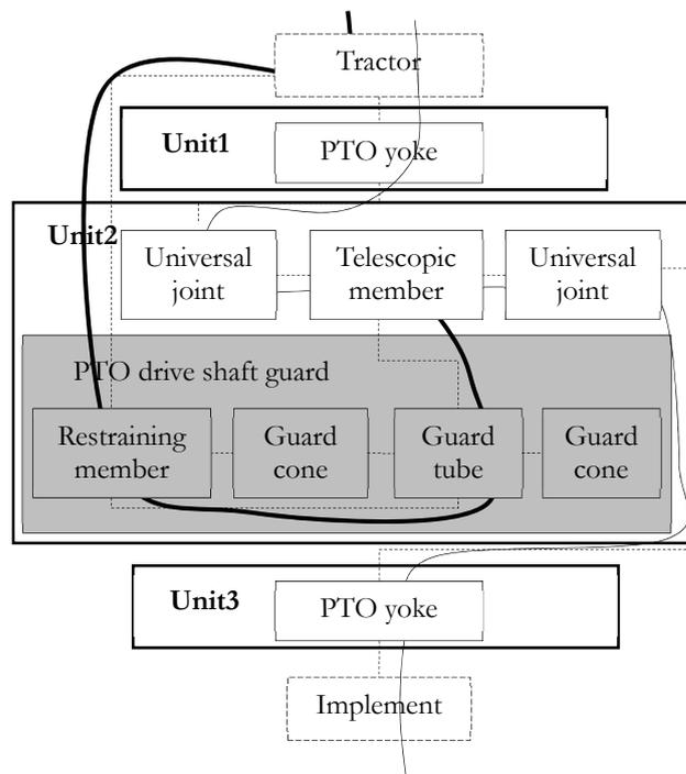
Figure 9. PTO system component interaction.
