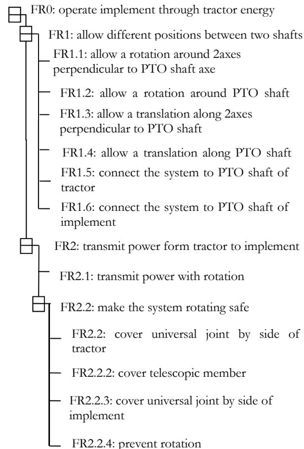
Figure 11. DPs and FRs hierarchies of a PTO system.
