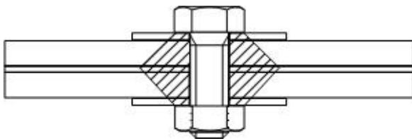
Figure 7. Zone in compression under bolt pretension using a flat washer.
