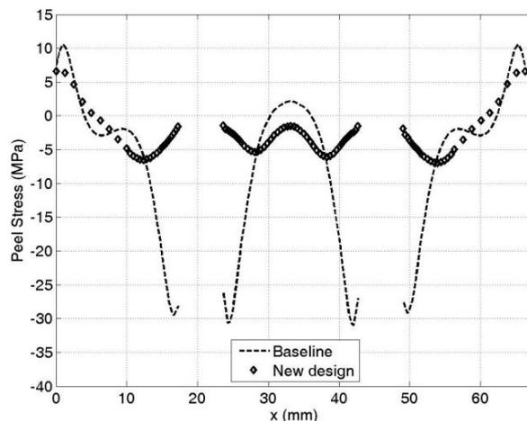
Figure 13. Comparison of the adhesive peel stress (measured in the middle plan of the joint).
