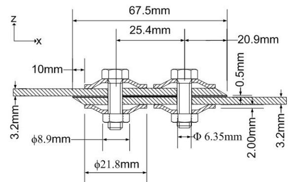
Figure 10. Dimensions of the new joint geometry analysed.
