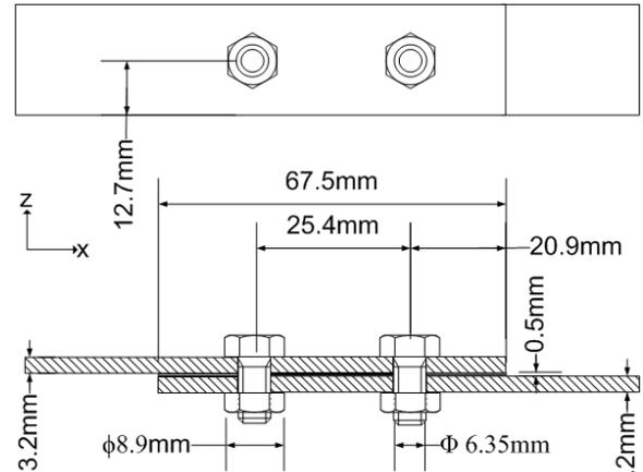
Figure 9. Dimensions of the baseline geometry analysed.
