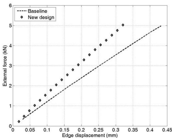
Figure 11. Comparison of the joints rigidity.
