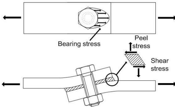
**Figure 1. Principal stress in a single-lap hybrid joint.**
