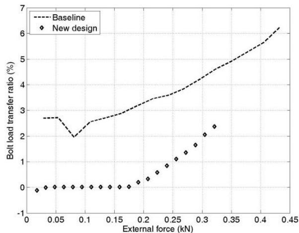
Figure 12. Comparison of the bolt load transfer ratio.
