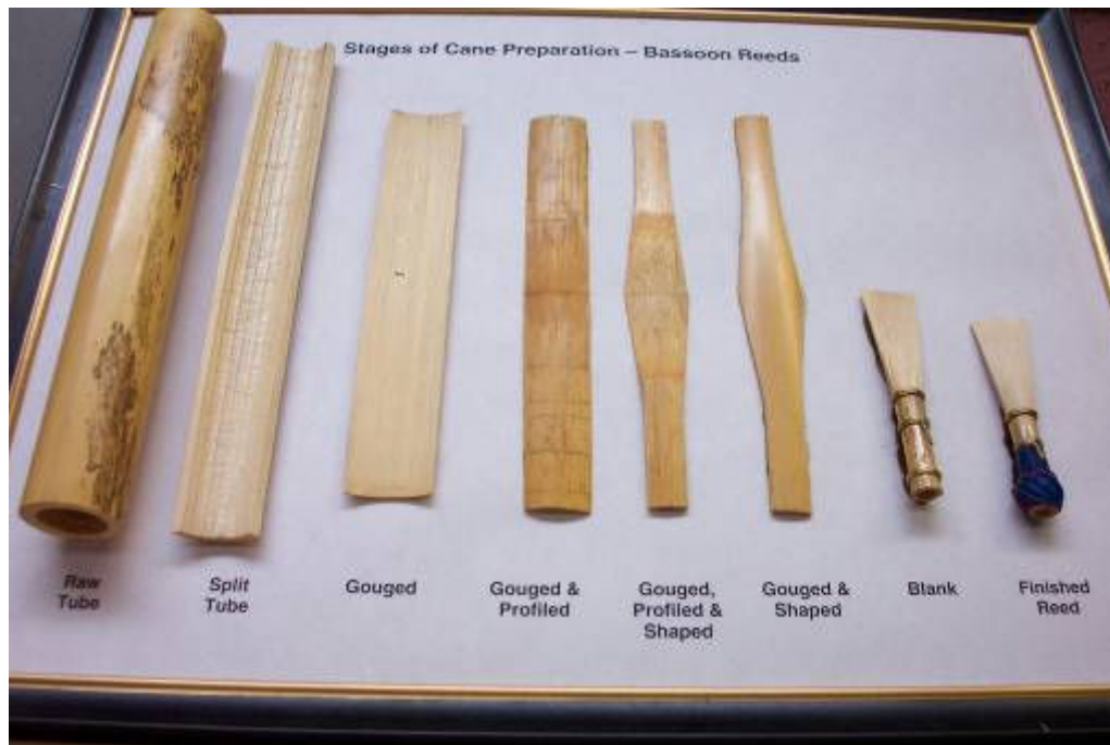
Figure 2. Stages of Preparation for Bassoon Reeds
