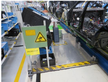
Fig. 4. Example of a mobile platform for final assembly.
